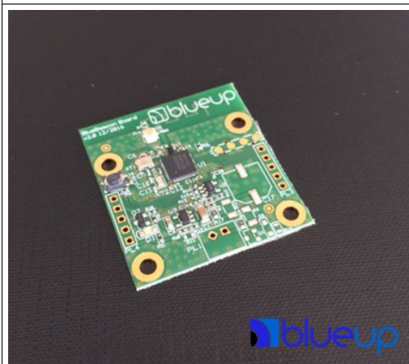
BlueBeacon Board OEM: UFL connector for external antenna
