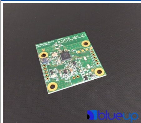
BlueBeacon Board OEM: integrated antenna
