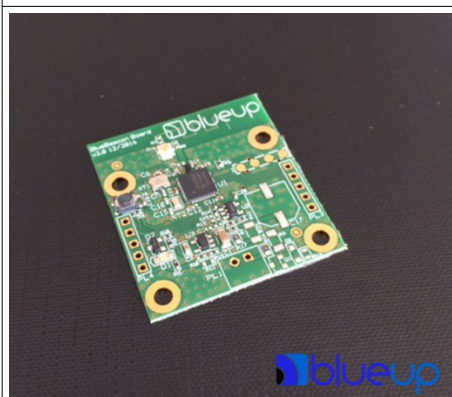
BlueBeacon Board OEM: UFL connector for external antenna
